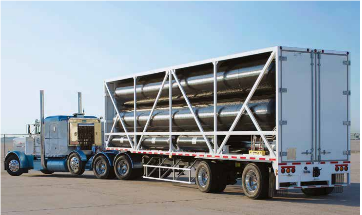
Hexagon's TITAN® cylinders are the largest all-composite commercial pressure vessels in the world.
